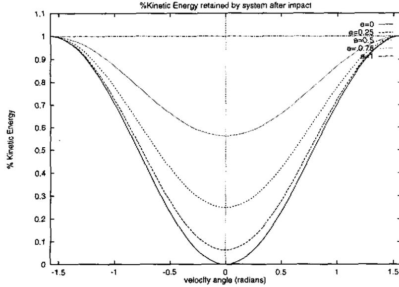
Figure 6.4: Percent of Kinetic Energy retained after collision
