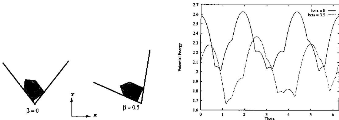
Figure 2.3: left: A part held in two palms, at two different palm orientations (but the same relative angle between the palms). right: The curves in the  $(\theta, y)$  plane describing the poses of the part in contact with both palms simultaneously.
