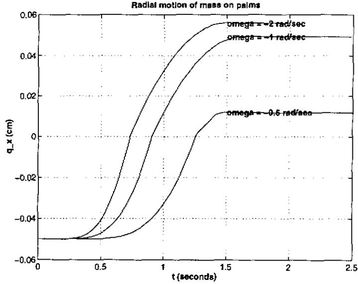
Figure 6.7: Radial motion of a point mass on a cone with  $\phi = 2.1588$ , tilting clockwise at -2, -1, and -0.5 rad/sec respectively. In each case the mass starts at rest on a horizontal left palm, 5 centimeters from the cone vertex.
