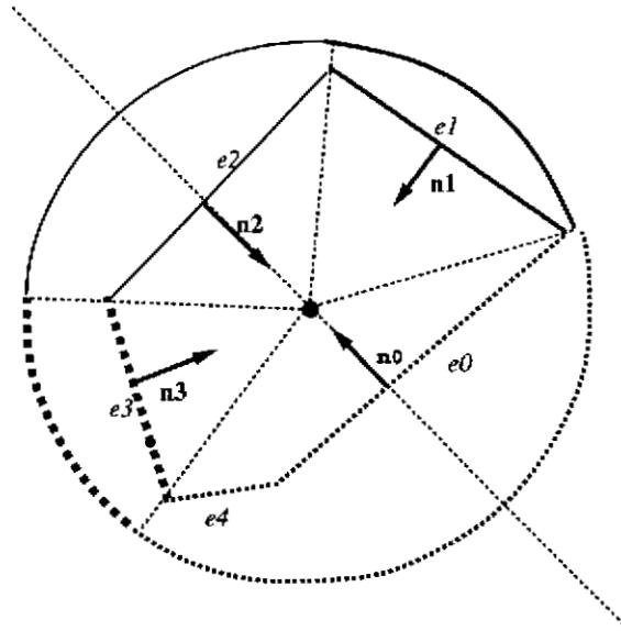
Figure 7.14: If  $P$  is resting on edge  $e_0$  on the left palm, it can reach edges  $e_1$  or  $e_2$  on the right palm by a clockwise tilt. If  $P$  is resting on edge  $e_1$  on the right palm, it can reach edges  $e_3$  or  $e_2$  on the left palm by a counterclockwise tilt.
