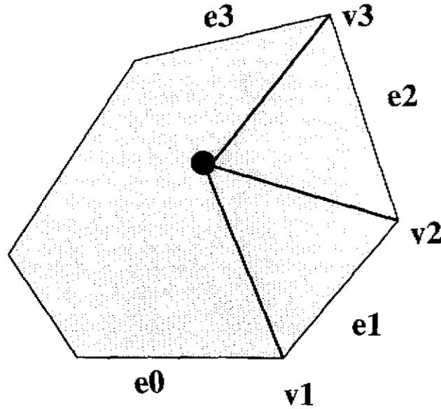
Figure 7.11: If edge  $e_0$  is resting on the left palm, then the vectors  $\mathbf{v}_i$  formed at vertices  $v_1$ ,  $v_2$ , and  $v_3$  form strictly acute angles with  $e_0$ . Hence, there are pure tilt motions to transfer the part to one of edges  $e_1$ ,  $e_2$ , or  $e_3$  on the right palm.
