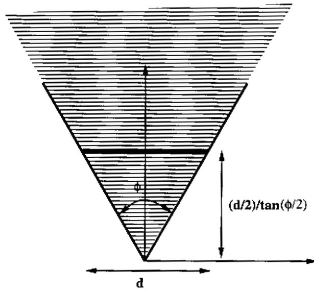
Figure A.1: The shaded portion shows the range of locations of the center of gravity satisfying the conditions of Theorem 17.
