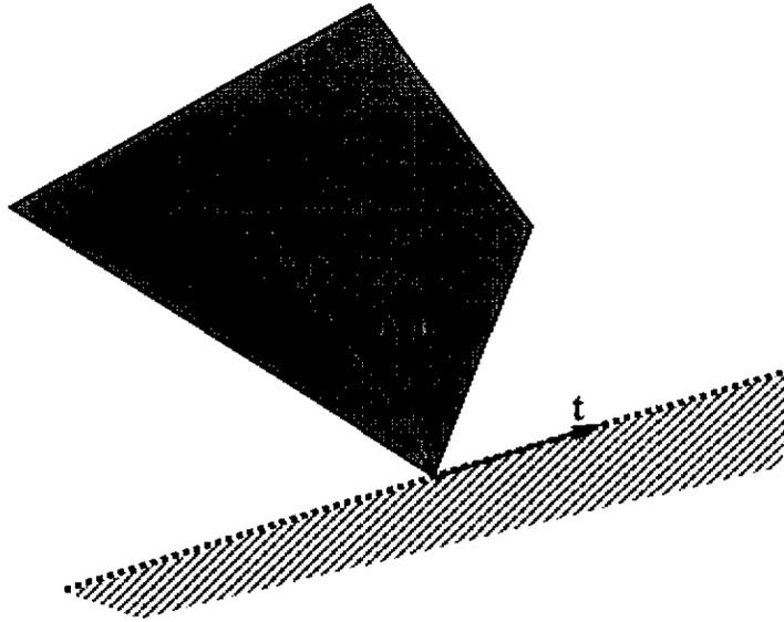
Figure 2.4: Object making point contact with an obstacle
