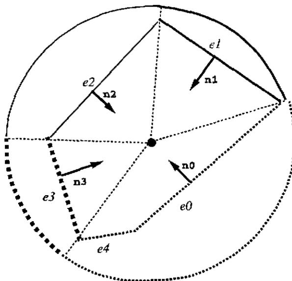
Figure 7.13: Construction for determining reachable edges. Note that edges  $e_0$  and  $e_4$  correspond to the same arc on the circle. This is because edge  $e_0$  is the stable edge to which the unstable edge  $e_4$  will fall.
