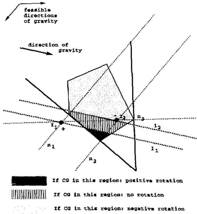
Figure 7.10: Determining the rotation sense of a part
