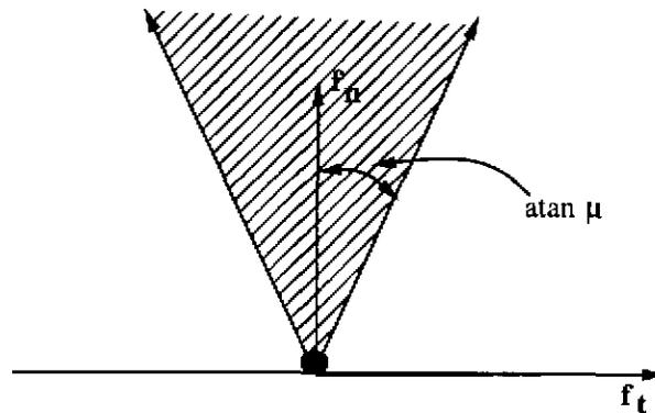
Figure 2.5: Friction cone of point mass on palm
